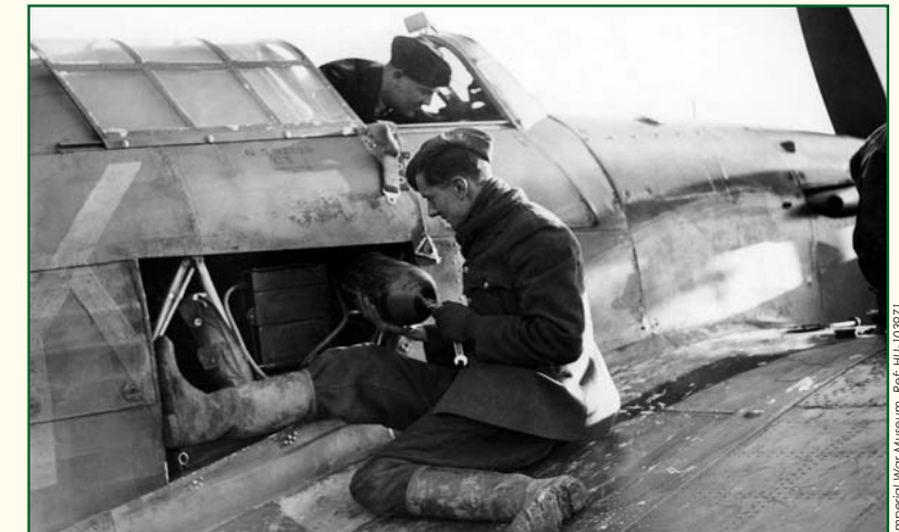
Instruments are cleaned and the oxygen cylinder replaced before the next flight, 30th November 1940.
